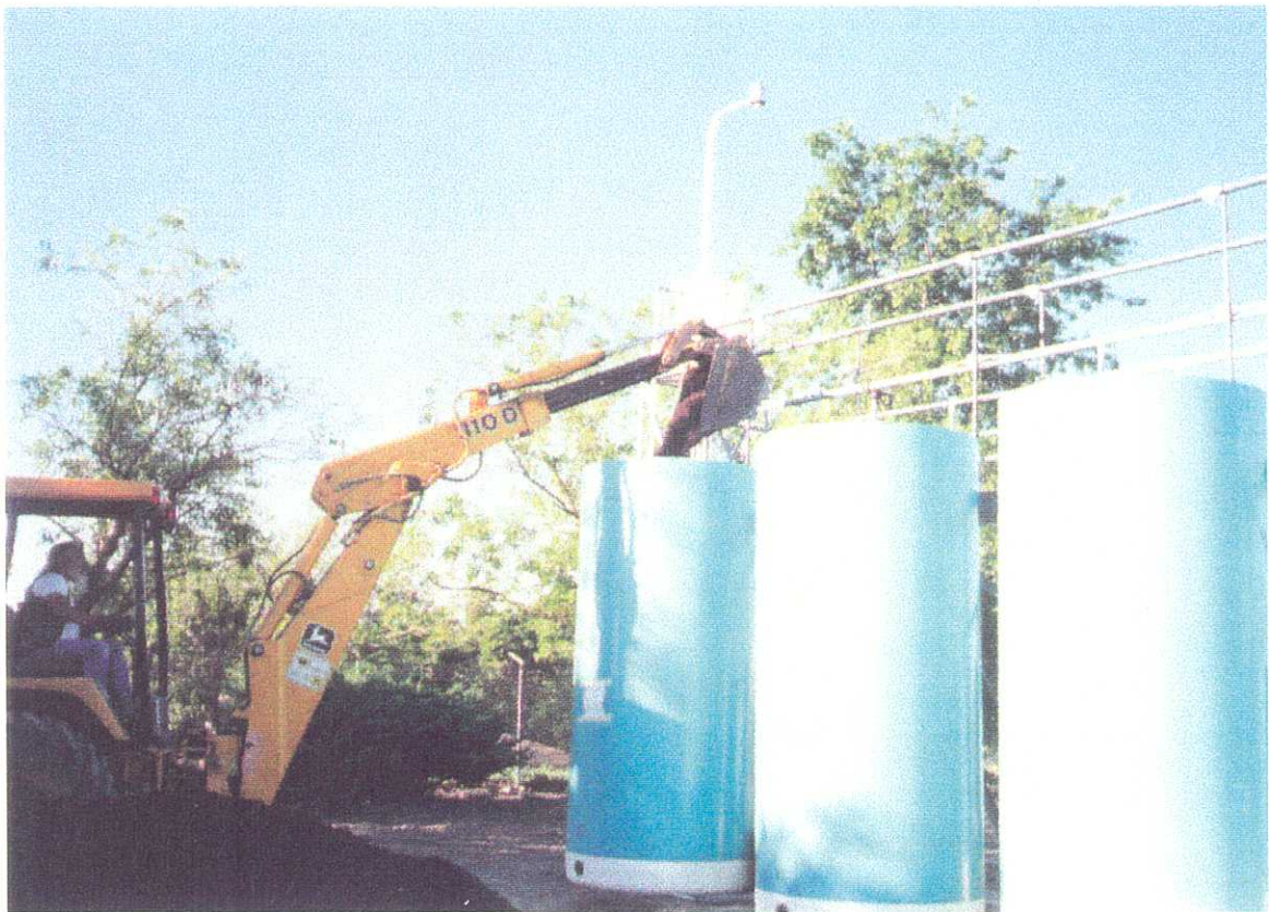
The peat soil was mixed by a backhoe prior to loading into the tanks.
